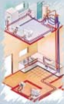
Flexible PEX pipe in conduit with unvented mains pressure cylinder.
