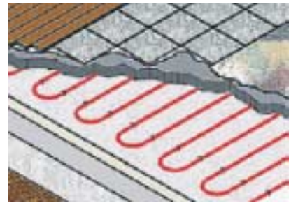
Pexatherm-e cable stapled to Multiboard-e insulation in screed under any floor finish.
